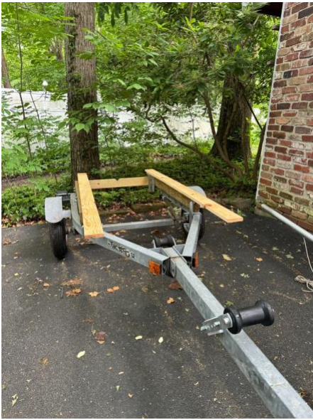
Figure 3 Laying out lumber for bunks.
